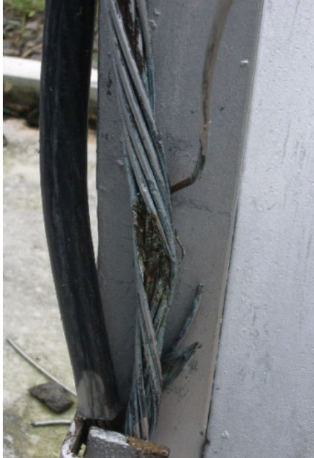
Biñan – (1) Frayed conductor; and (2) melted conductor
